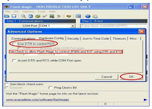
Uncheck the box which is highlighted to don't allow Flash Magic to control PSEN & RST using DTR & RTS. Now go for Communication selection, select 'COM 1' from 'COM PORT' Option if you are using serial port. If you are using USB to serial converter then find out COM port number with the help of documentation provided with the USB to serial converter.
