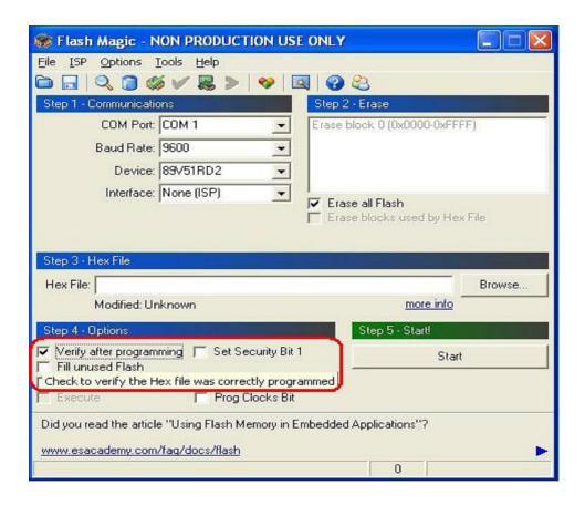
After doing all the required settings, connect serial cable between Controller Board and PC. Turn on the Board and click on the **Start**', it will ask to '**RESET TO DEVICE IN TO ISP MODE**', now press RESET Switch on the Controller Board, Flash magic will load hex file on the robot and verify it for correctness.
